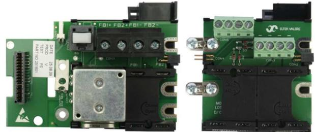
Plug-in battery and load breaker
