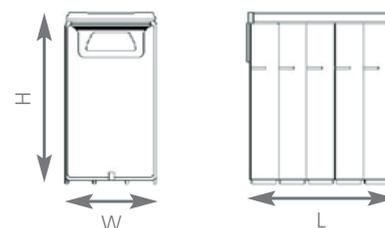
The block length and weight are determined by the number of cells in the block. All tabulated dimensions are maximum values.
